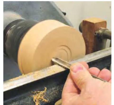
▲ Pic.6 To be able to turn the top detail you need a way of turning it around. Turn a dovetail chucking recess in the bottom to suit your chuck. If you make this 3mm deep, it can be filled with a piece of hardboard before you apply the baize
